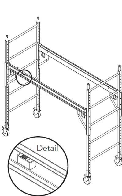
3) Attach the second arm brace as described in step 2. Make sure both arm braces are positioned at the same level. Be sure the platform hold down devices are turned out of the way.
