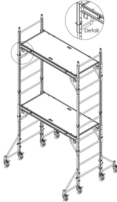
10) Lay a plywood platform on the braces. Then line up the four holes in the plywood with the pins on the arm braces. Turn the platform hold down devices so they "trap" the platform onto the braces. Secure the braces using 2" snap pins through the "U" channel and the frames.
