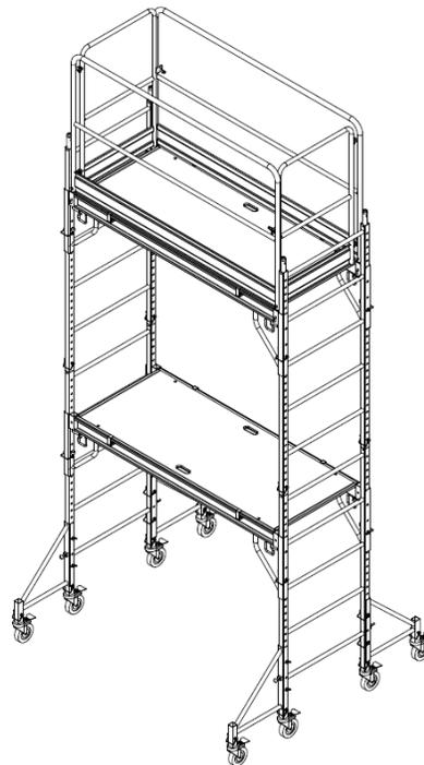
12) Set the guard rail panel (toeboards are attached to guard rail) on the second level arm brace and secure with 2" hinge pins. Repeat to install the second piece of guard rail to the unit.
