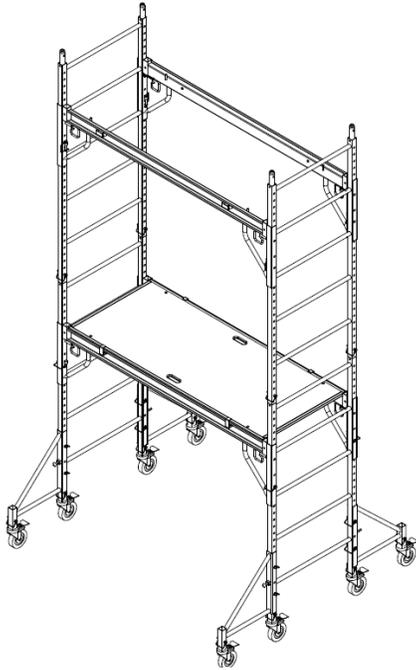
9) Attach the second level arm braces, one at a time, as described in Step 2 and position them to the desired location on the second level ladder frames.
