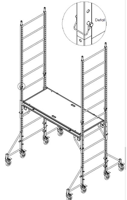
7) Attach the remaining three outriggers as described in step 6. Make sure that the casters on the outriggers are level with the casters on the ladder frames.
