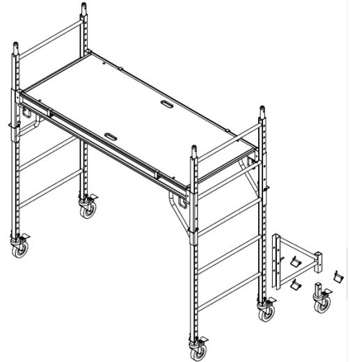
5) Optional: For additional security insert 2" snap pins through the "U" channel and frames after the platform height has been properly set.
