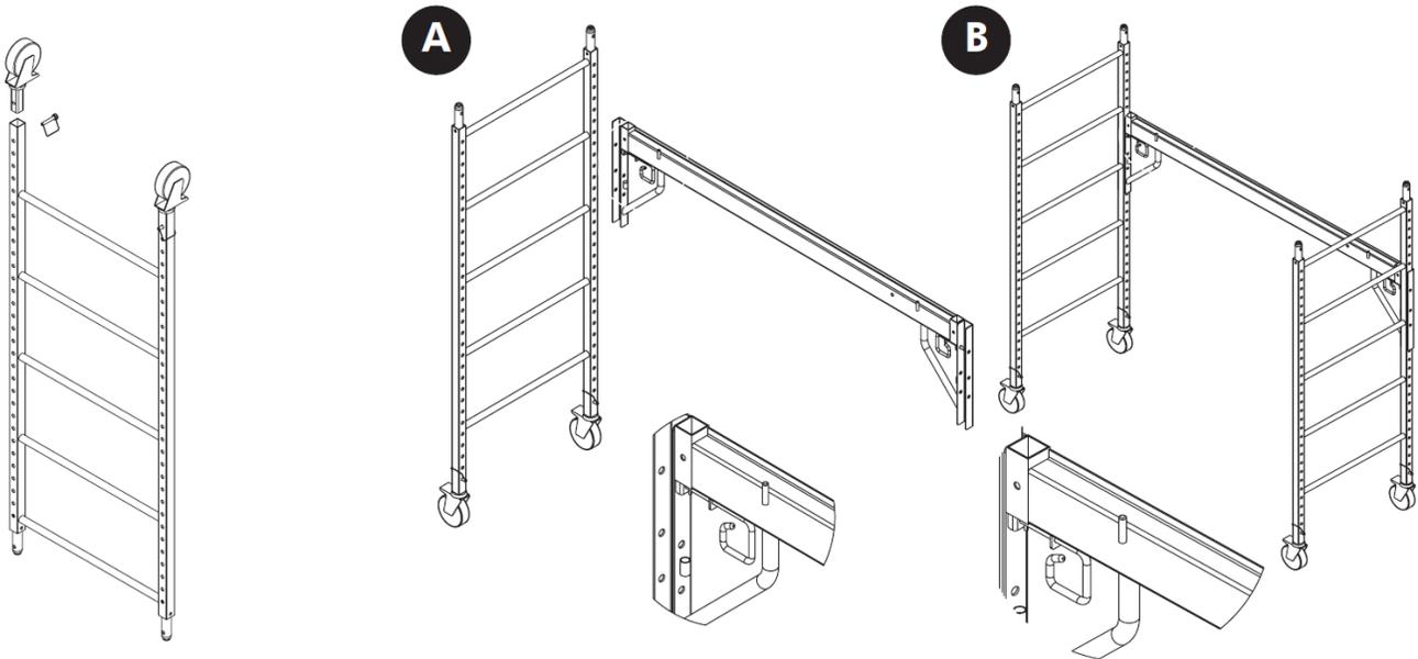
1) Turn the end frames upside down and insert the casters into the frame legs. Pin the casters in place with 2" snap pins.
