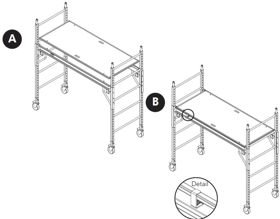
4)(A) Then lay a plywood platform on the braces. Line up the 4 holes in the plywood with the pins on the arm braces. (B) Turn the platform hold down devices so that they "trap" the platform onto the braces.
